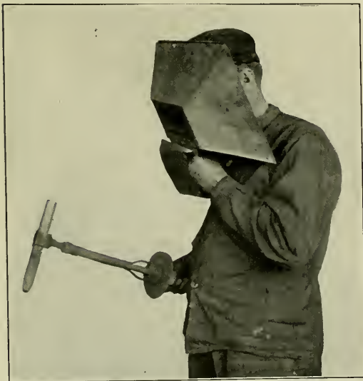
Graphite Electrode Holder and Hand Shield.
